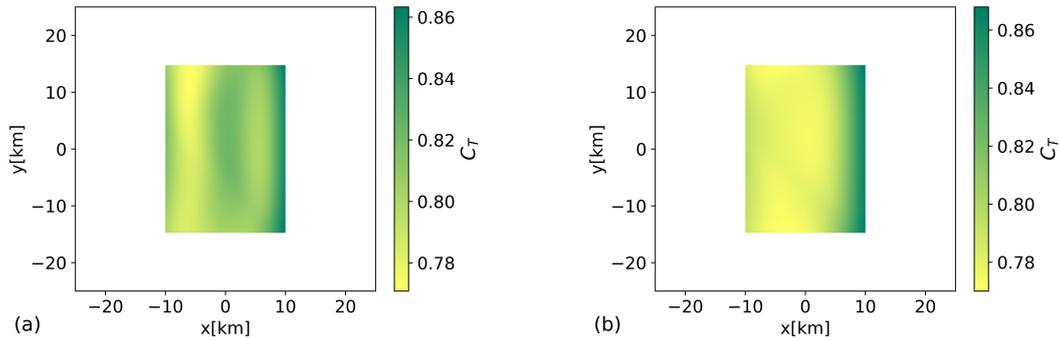
Figure 1: Planform view of (a) optimal turbine thrust coefficient space distribution in sub-critical condition ( $F_r = 0.9$ ) and (b) in super-critical condition ( $F_r = 1.1$ ). The length and width of the wind-farm is 20 and 30 km, respectively.
