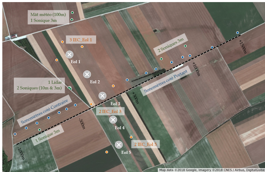
Figure 1 Campaign site presenting the wind turbines and the acquisition devices (sonometers in blue, meteorological devices in green and acoustic power measurement in orange).
